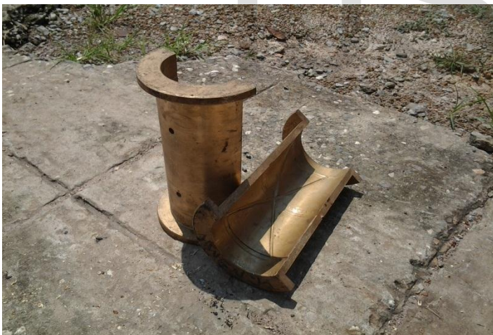
Fig. 1.1: Scrap flange sleeve bearing used as raw material at Fox Foundry, Kitwe (February, 2014)
