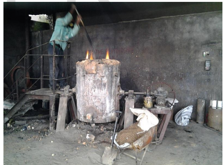
Fig.2.1: Melting of bronze in progress at Fox Foundry, Kitwe (February, 2014)
