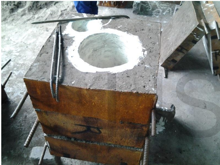
Fig.2.2: Mould prepared for a secondary crusher counter-shaft bearing billet at Fox Foundry (February, 2014)
